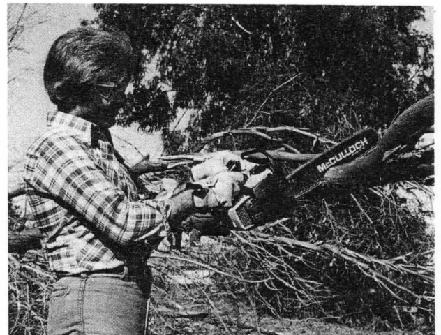
Figure 9-33. A chainsaw needs a diaphragm carburetor so it can work in all positions. (McCulloch Corp.)
